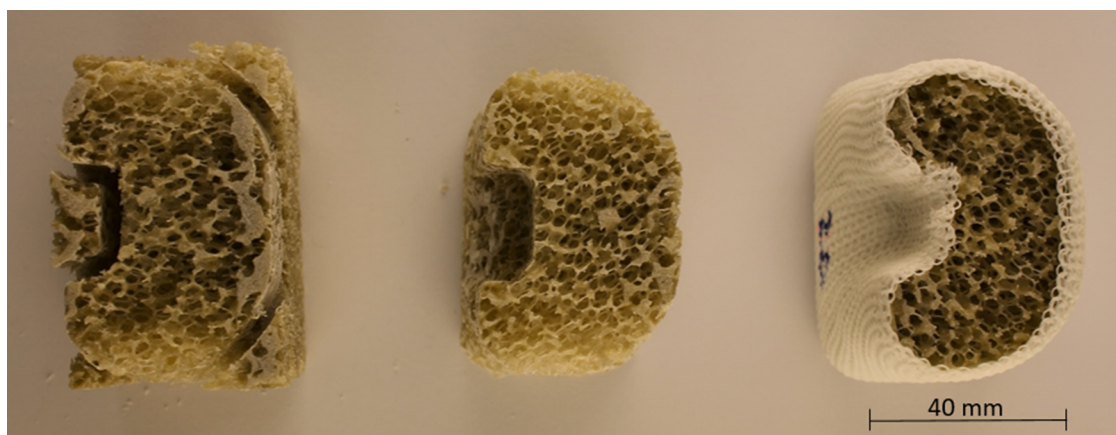
Fig. 1. Left: Milled model with protruding edges. Middle: Model with broken edges. Right: Model with wrapped Cellacast® as cortical bone.
